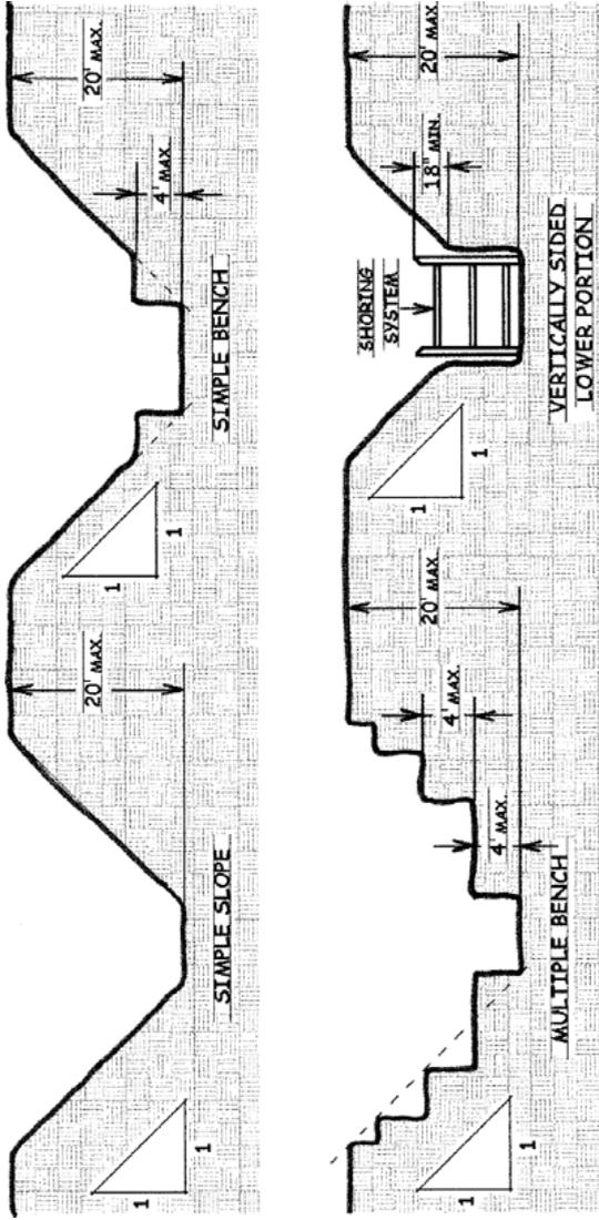
Illustration 8 | Benching & Sloping For Excavations Made in Type "C" Soil
